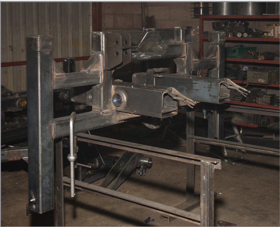
WORK ON another Bryce Suma post driver in progress in the workshop Ref:RH191217012
