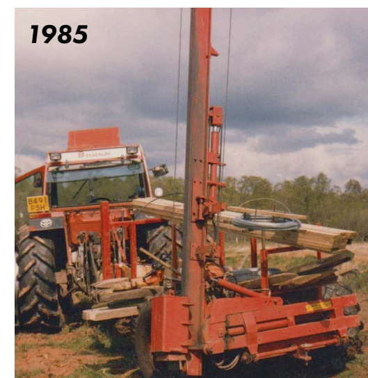
'My powered axle design which included sideshift and backshift. Note double slider sideshift. A Bryce mast was fitted later.'
