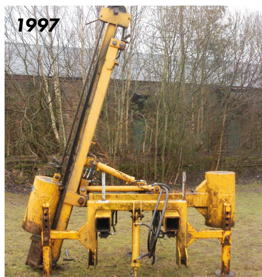
'The first tractor mounted Bryce Profi I introduced to the marketplace. This included sideshift and backshift like the trailed machine on the left.'
