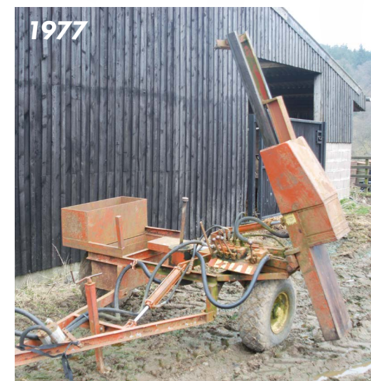
'I purchased 2 Linden Post Drivers. Modifications included combine wheels, box for wire coils and hydraulic jack leg behind the counter balance.'
