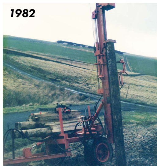
'I then made a heavy duty version with 26ply aircraft tyres to stop bounce, a frame for carrying materials and I used a Kinghitter Mast with 700lb hammer.'
