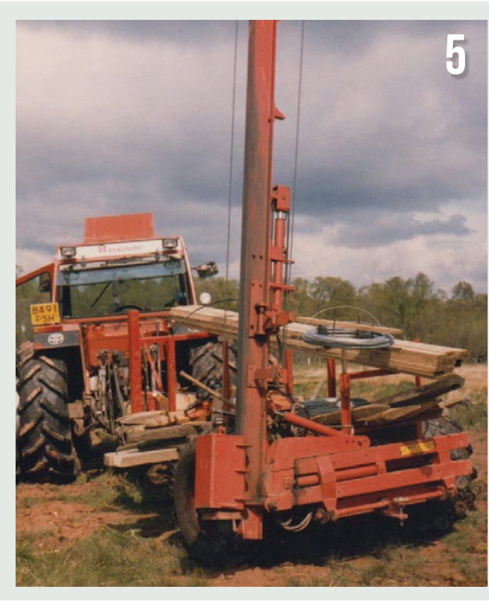
THE 6 WHEEL DRIVE OUTFIT MADE IN 1985. NOTICE THE DOUBLE-SLIDER SIDESHIFT, AND MAST TILT RAM BRACKET WHICH MANY YEARS LATER WERE INTRODUCED ON THE BRYCE SUMA PROFI.
